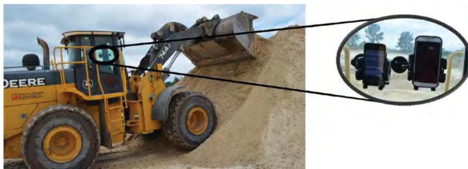
Figure 2. Smartphones mounted inside the front-end loader cabin
