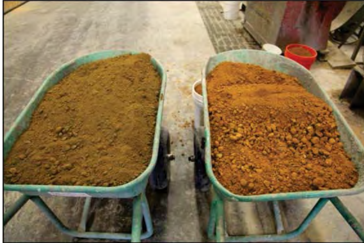
Figure 5. Louisiana clay before (right) and after (left) adding 7% portland cement by vol.
