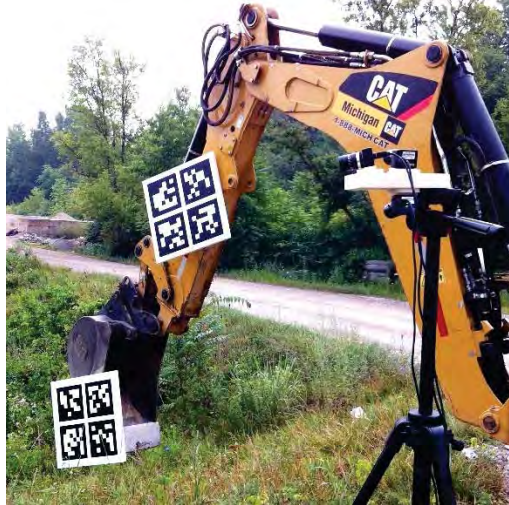
Figure 16. Calibration of cable potentiometer prototype installed on a backhoe
