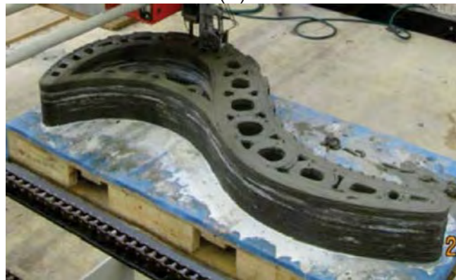
Figure 2 – Complex Concrete Printing Product (a) 3D Model (Lim et al. 2012), (b) During printing (Le et al. 2012)
